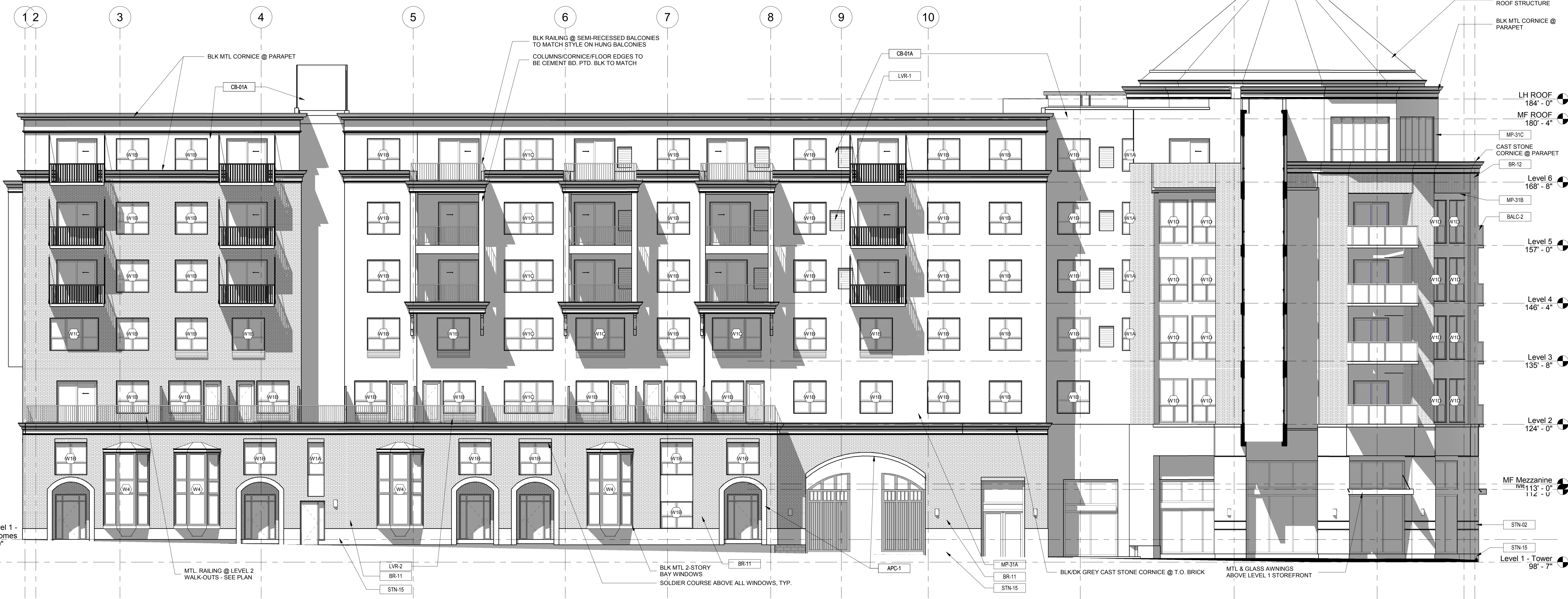
1 EAST ELEVATION @ BRIDGE A300B 1/8" = 1'-0"
